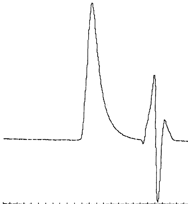
Figure 1. GPC plot of polymer I-5 in THF at 50 °C.
